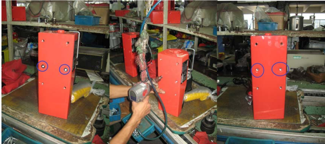
Step 1: release the two screws shown in the blue circle.
