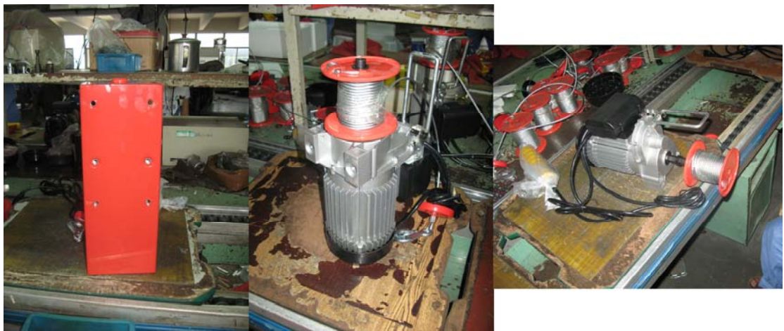
Step 2: remove the red bracket of the electric hoist and take the rope drum out
