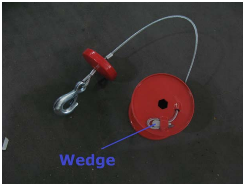
Step 3: remove the wedge from the red rope drum, then you can take the broken steel rope out.
